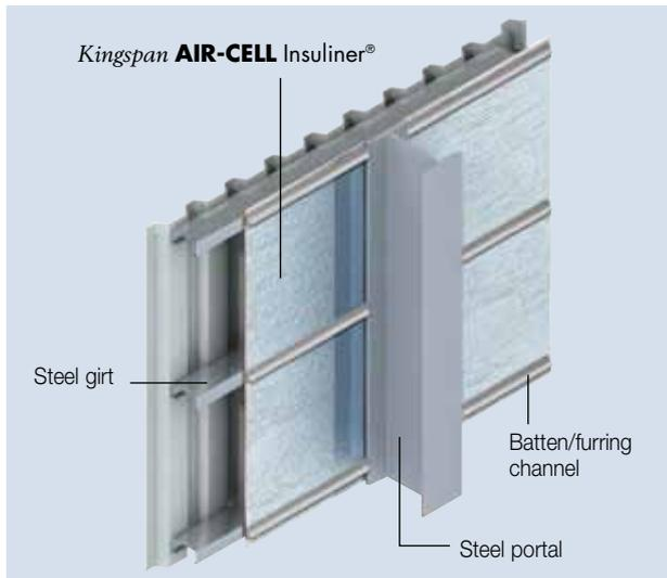
Figure 7 Warehouse wall retrofit installation
