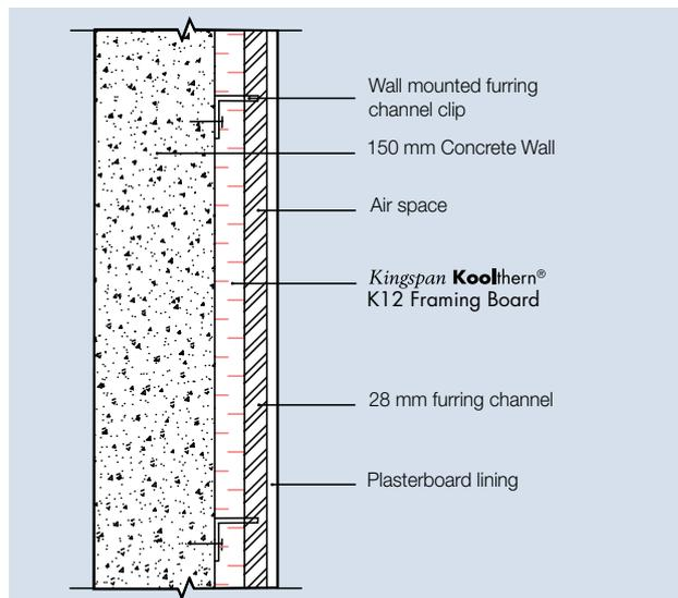
Figure 6 Side elevation of *Kingspan Kooltherm*<sup>®</sup> K12 Framing Board clip-and-channel system
