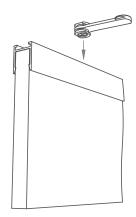
Once the connector clips are turned 90 degrees, the Frontier Channel can be disconnected from the ceiling.
