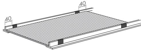
On the final row select an ambiguous position to leave a tile unclipped as this will allow access to the ceiling cavity.
