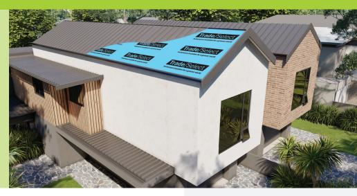
Trade Select™ Sarking is a Heavy Duty radiant barrier, designed for multi-purpose use as both roof sarking and a wall wrap. The reflective foil side provides Thermal Control and extra R-value when installed facing an air cavity. The multi-layer structure provides superior strength, flexibility, and durability. Classified as a Water Barrier and Class 2 Vapour Barrier, Trade Select™ Sarking acts as a barrier to air, radiant heat, moisture ingress and dust penetration.
