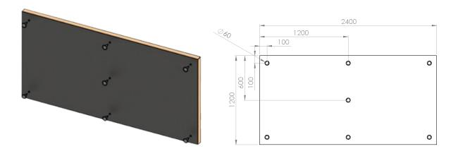
When fixing the panel to the soffit, start with the centre fixing, this will help support the weight of the board while the remaining fixings are installed.
