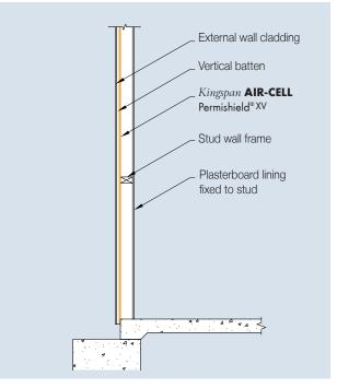
Figure 6 Side elevation of  $\mathit{Kingspan}$  AIR-CELL  $\mathsf{Permishield}^{\otimes}$  XV on timber-framed wall
