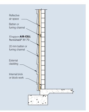
Figure 2 Side elevation of  $\mathit{Kingspan}$  AIR-CELL  $\mathsf{Permishield}^{\oplus}$  XV 70 in a reverse brick veneer wall
