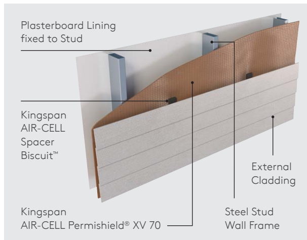
Figure 3. Kingspan AIR-CELL Permishield® XV 70 on a steel-framed wall.
